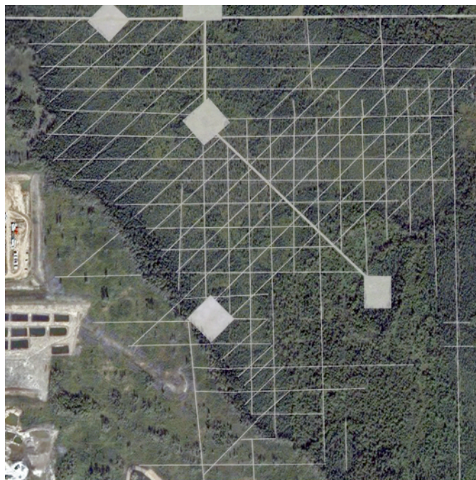
Figure 22. Aerial Photograph of OPTI/Nexen Long Lake SAGD Facility. Note facility construction at left. Adobe Photoshop used to highlight 93 visible seismic features. Photograph is 1km x 1km. (Source: Google Earth)
